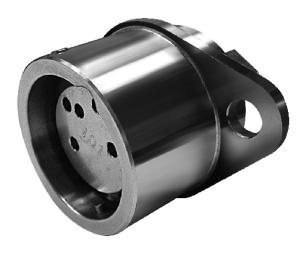
The HD Series Type SA1 and SA2 switchgear adapter interlocks have a 3/8" (9.5mm) square, 7/8" (22mm) long shaft that is controlled by the robust HD Series key. The mounting flange will accept two 1/4" (7mm) mounting bolts. Type SA1 and SA2 interlocks can be ordered with the shaft rotating clockwise or counterclockwise. Multiple degrees of rotation are available also.
